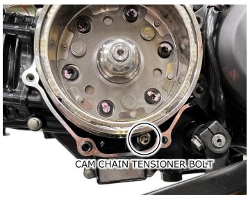
• Fix cam sprocket by using universal holder. Remove flange bolt, washer, then remove cam sprocket by camshaft, and remove cam chain from cam sprocket.
