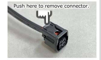
• Remove EOT(oil temperature sensor)/sensor guard, etc.
