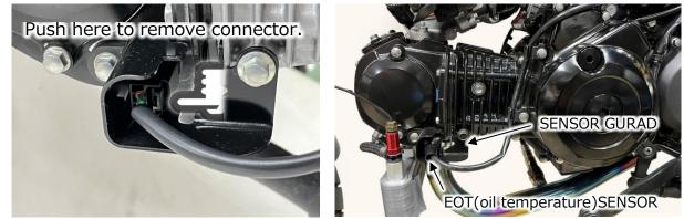
• Remove AC generator 2P connecter/CKP sensor bullet terminal.
