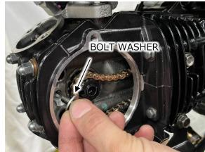
Remove cam shaft. Turn cam shaft key groove 45° to IN side to pull, then turn 45° to EX side to pull. Hold not to hang rocker arm to cam nod.
