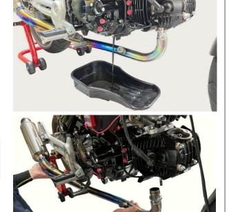
• Remove O2 sensor / sensor guard / plug cap, etc.
