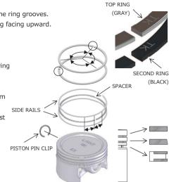
After installation, the piston rings should be free to rotate in the grooves.
